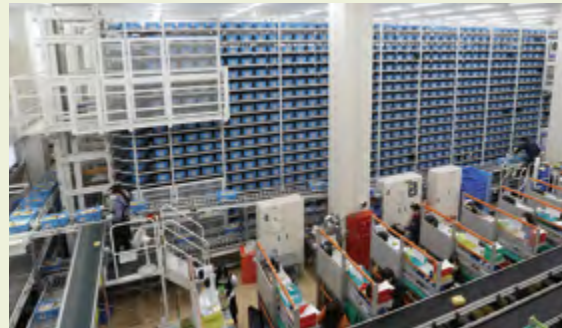
Rotary Rack H (built for use at SUNCO INDUSTRIES CO., LTD.)
